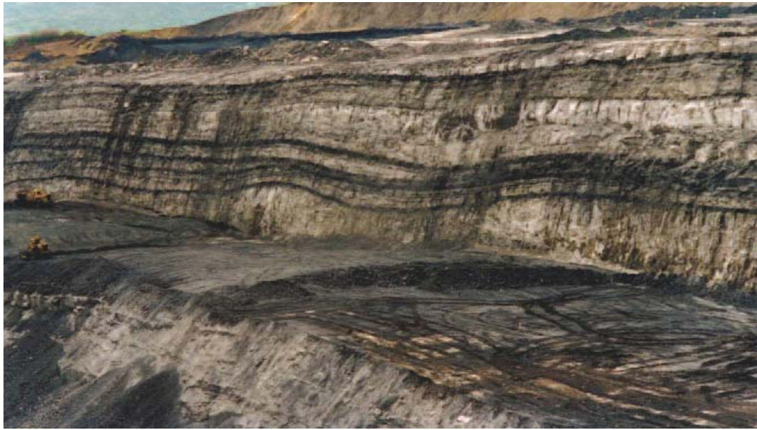
Cretaceous coal strata exposed in a bench cut of the Williams Fork Formation at the Kennecott Corp. Colowyo surface coal mine in Moffat County, Colorado. Note how the coal beds split and roll.
