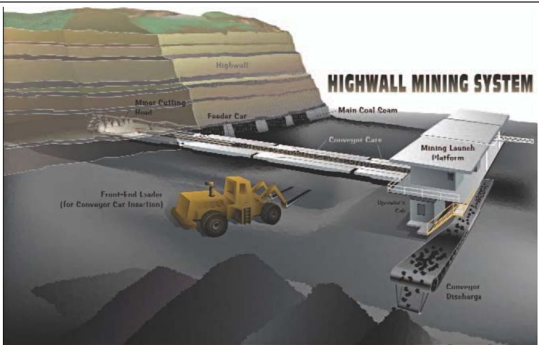
Block diagram of a highwall miner operating in cross-sectional view in a surface mine operation.
